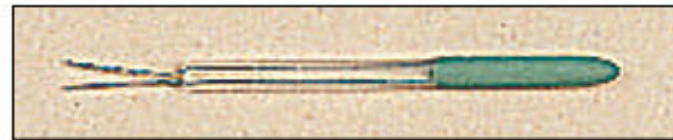
Glass sealed Bifilar Winding
